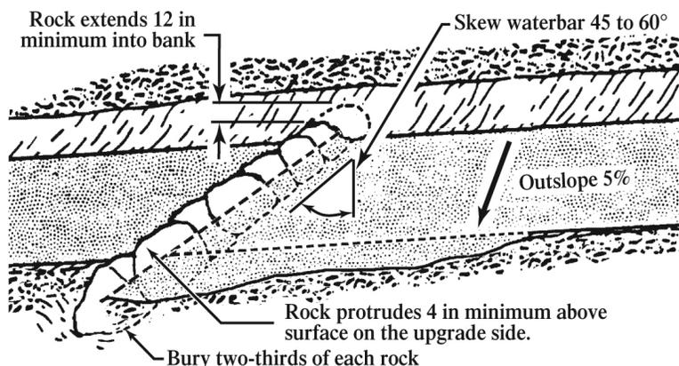
**Figure 2. Diagram of modern waterbar construction**
