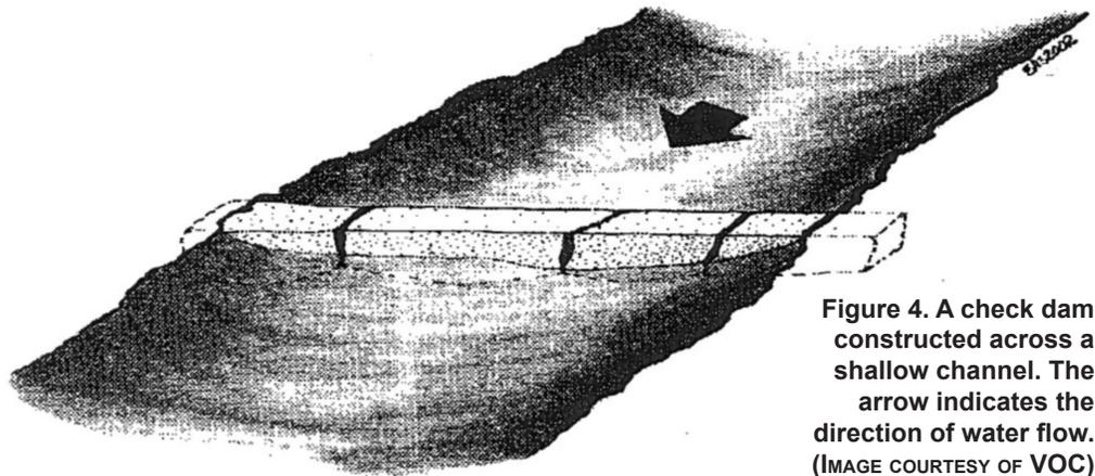
**Figure 4. A check dam constructed across a shallow channel. The arrow indicates the direction of water flow.**
