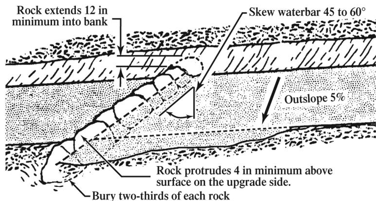
Contemporary waterbar design favored by PCTA is a broad earthen **drain dip**, reinforced at the the high point of the **backramp** with a completely buried log or line of tightly fitted large rocks. See diagrams and "Key Concepts" above for drain dip and waterbar specifications.
