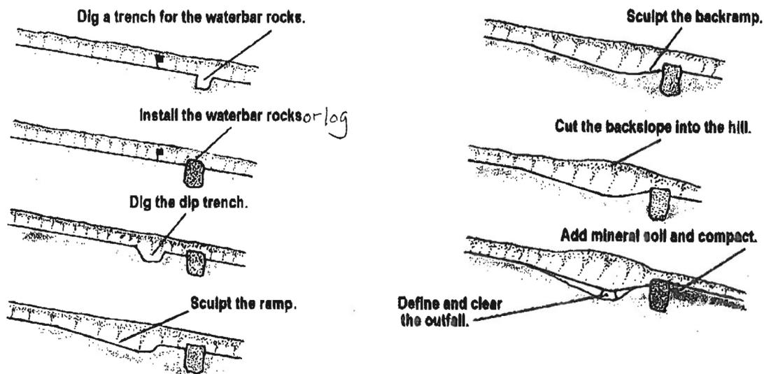
Pile and compact excavated soil on both sides of the bar to protect it from erosion. Bury log bars completely so they are just barely showing, insuring that water exits well before the bar. If there is excess dirt, look for cupped tread to fill down the trail from the drainage—never let good dirt go to waste.
