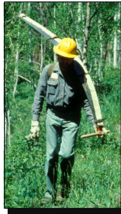
Figure 34—Transporting a crosscut saw to a jobsite by carrying the saw on the shoulder with the teeth facing outward. Saws need to be sheathed when they are carried for long distances.
