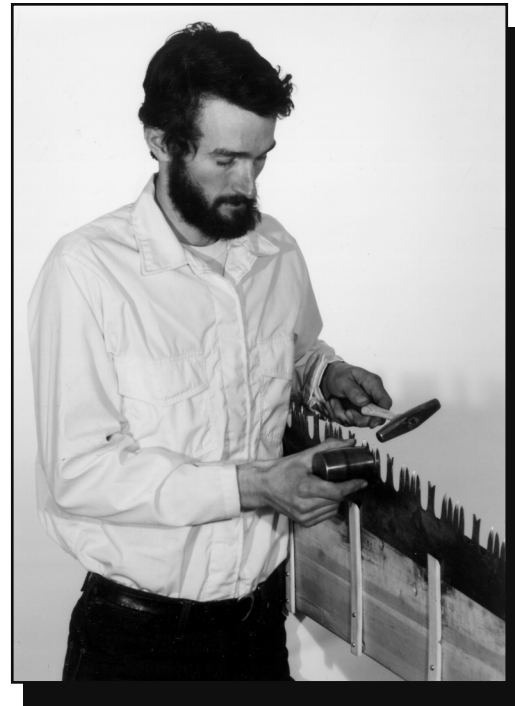
Figure 26—Warren Miller setting cutter teeth.
