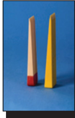
Figure 3-22—Double-taper wedges are designed to reduce bind.
