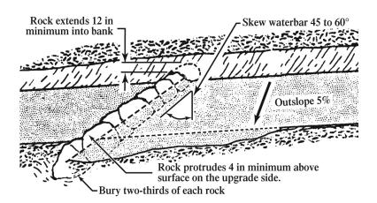
Contemporary waterbar design favored by PCTA is a broad earthen <u>drain dip</u>, reinforced at the the high point of the <u>backramp</u> with a completely buried log or line of tightly fitted large rocks. See diagrams and "Key Concepts" above for drain dip and waterbar specifications.
