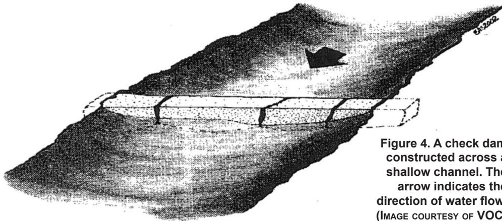
Figure 4. A check dam constructed across a shallow channel. The arrow indicates the direction of water flow. (IMAGE COURTESY OF VOC)
