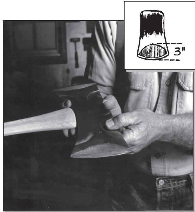
Figure 66—When sharpening, try for a fan-shaped effect on the cheek of the ax (drawing by Frederic H. Kock).
