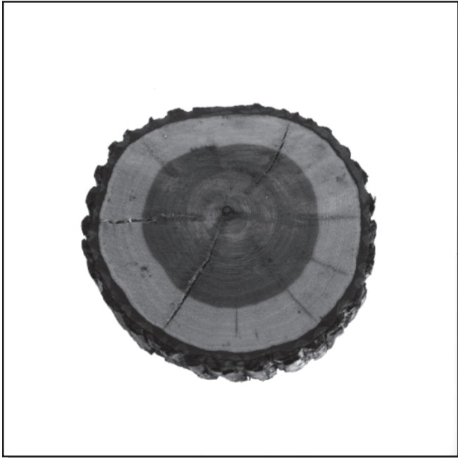
Figure 35—Hickory cross section. The outer, white sapwood makes the best ax handles. This particular piece is too small and too riddled with checks to be good handle stock.
