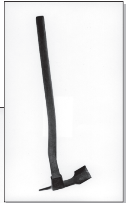
Figure 27a—Collins lipped shipwright's adz.
