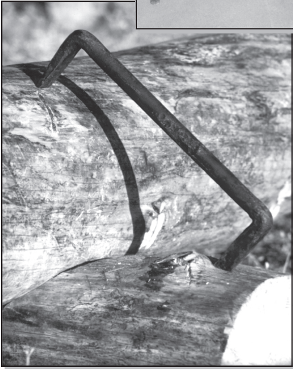
Figure 97—Use a log dog to secure the log to the yoke.
