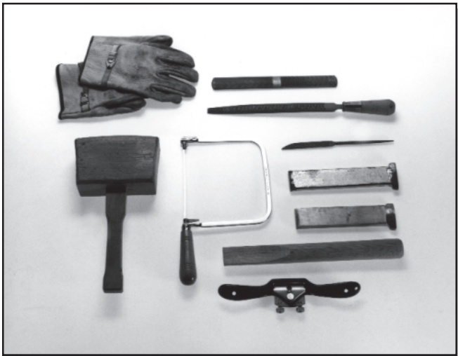
Figure 40—Tools needed for hanging an ax include (clockwise, from top left): leather gloves, four-in-hand rasp, wood rasp, keyhole rasp, steel drift for double-bit ax, steel drift for single-bit ax, hickory drift made from old handle, spokeshave, coping saw, and wooden mallet.
