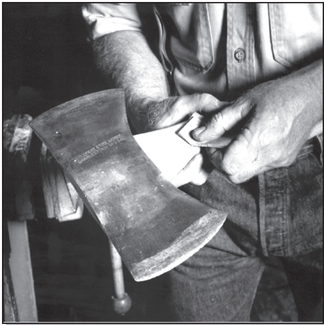
Figure 59—Sand any paint, varnish, shellac, or wax from the handle. Sand the handle smooth on all but 6 inches of the butt section. The body of the sanded handle is where your hand will slide. You don't want any splinters or rough wood there.
