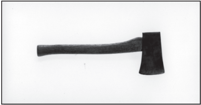
Figure 19—Plumb 2½-lb boy's ax with 19-inch handle—my favorite for log cabin work.
