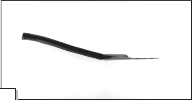
Figure 34b—A 19th-century S-bend broad ax handle.
