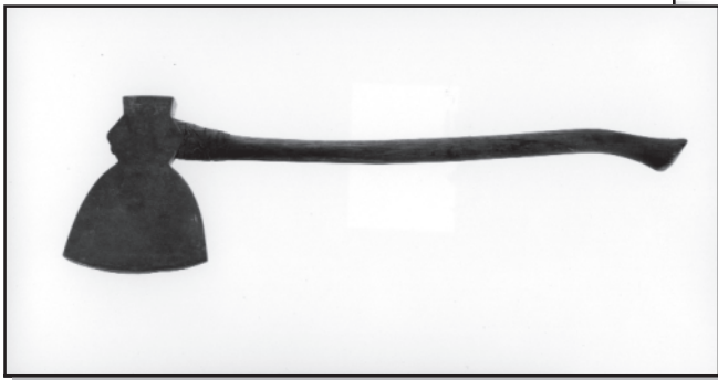
Figure 18e—A 19th-century shipwright's mast broad ax.
