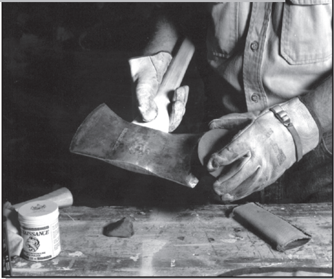
Figure 71—Use the ax stone in a circular motion, working into the edge, toward the middle of the ax head (drawings by Frederic H. Kock).
