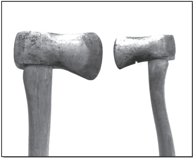
Figure 12—Winchester ax and hatchet, Michigan pattern, typical of the American felling ax.
