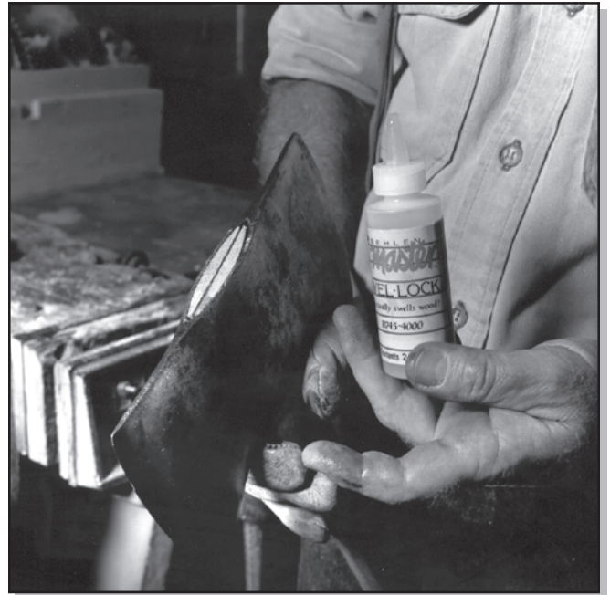
Figure 57—Before inserting the wedge in the handle, apply a coat of Swel-Lock to the inside kerf cut and the new wooden wedge. Swel-Lock is a product that swells wood. It is not a glue or an adhesive; rather, it penetrates and expands wood fibers to keep the new handle tight.
