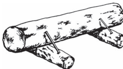
Figure 99—The chalk line will mark the top side of the hewn surface.
