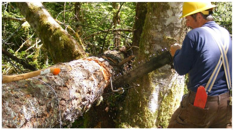
Install the underbucker on the side of the log that will not drop when the cut releases
