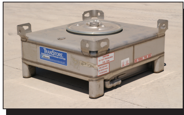
Figure 91—A 240-gallon DOT-406 tank being used to mix gelled fuel.
