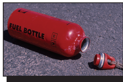
Figure 77—An aluminum fuel bottle that failed because it was overfilled.
