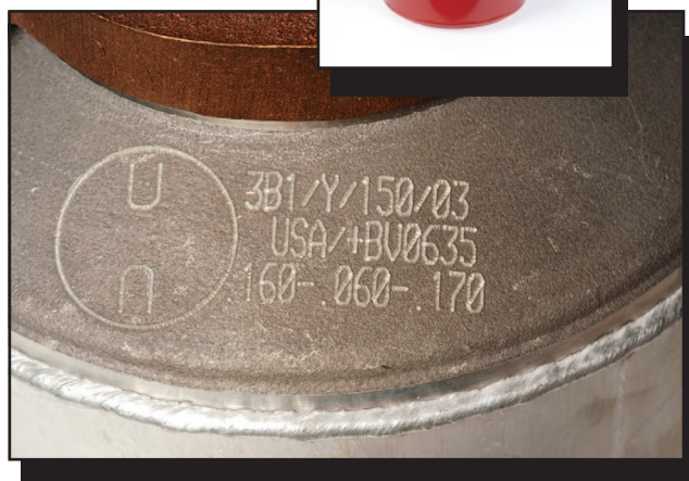
Figure 17—The UN marking shows that this drip torch meets DOT specifications.
