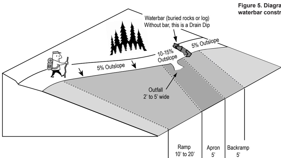
Figure 5. Diagram of modern waterbar construction
