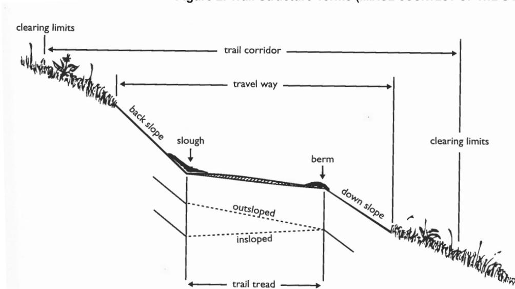
Figure 3. If your ankles start to roll, the tread has too much outslope. (IMAGE COURTESY OF USFS)
