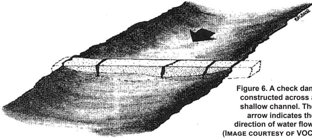
Figure 6. A check dam constructed across a shallow channel. The arrow indicates the direction of water flow. (IMAGE COURTESY OF VOC)
