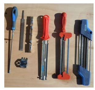
Round file, raker file, depth gauge, roller guide, file guide, file guide with raker file (single & dual side)
