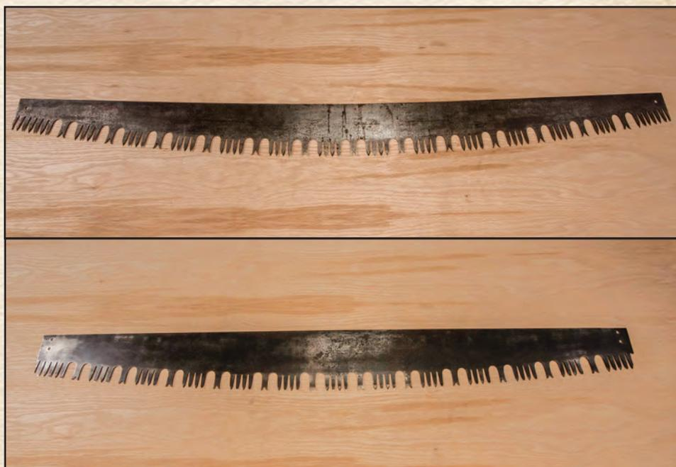
Figure 11-46—A felling saw (top) and a bucking saw (bottom).
