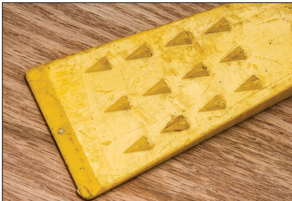
Figure 11-54—A wedge with a ridged surface.
