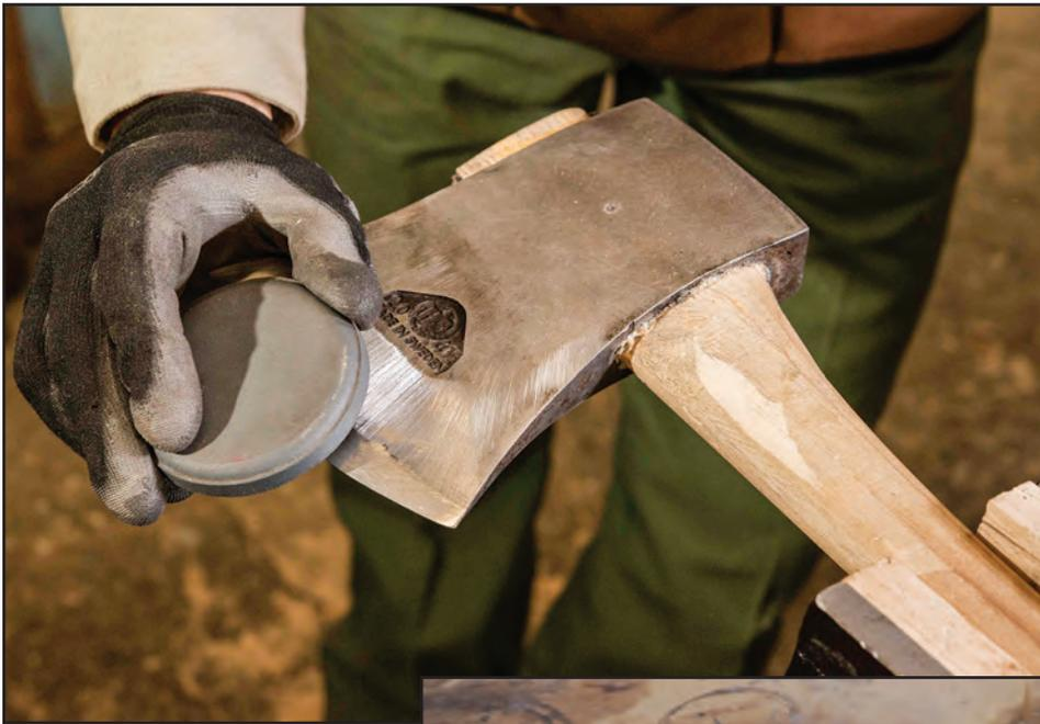
Figure 8–31 — Using an ax stone to hone the bevel.
