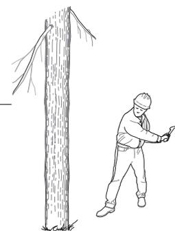
If you cannot easily remove an ax from a round of wood, use another ax or a maul and wedge to split the round and free the ax (figure 11-75).
