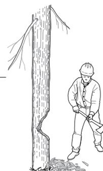
Felling techniques when using an ax and crosscut saw together are essentially the same as when using an ax alone. Use the crosscut saw to make a horizontal undercut about one quarter the diameter of the tree and use the ax to make a sloping cut that meets up with the horizontal cut.
