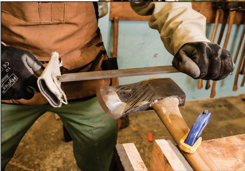
Figure 8–27—Lifting the file off the ax head at the end of the push stroke.
