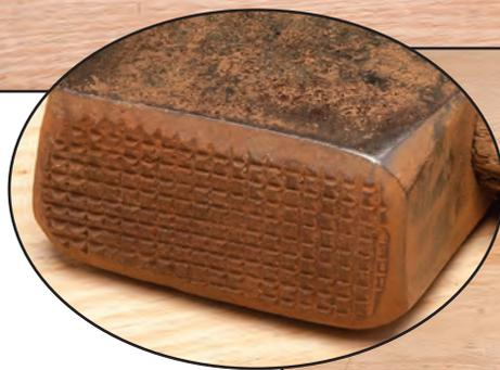
Figure 5-3—Plumb 5-pound and 3½-pound rafting-pattern axes with elongated polls. The inset shows a rafting-pattern ax with a waffled poll.
