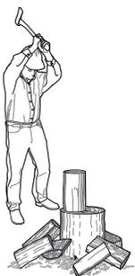
If the ax sticks in the round of wood, be careful not to apply too much continuous force trying to free it. Applying too much continuous force may result in a broken ax handle.
