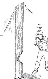
When using an ax and crosscut saw, it is best to use your ax to clear away the bark from the area you intend to cut (figure 11–49). The bark of a tree holds dirt, which can quickly dull a crosscut saw. Clearing the bark helps keep the saw sharp and cutting well. A sharp, well-tuned crosscut saw is easy to use. Sharpening a crosscut saw is time consuming; it is an art unto itself.
