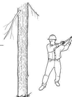
Ensure that the ax head and handle are tight. If the head becomes loose, you may be tempted to soak the ax in water to make the handle swell. This temporary fix is ill advised. As the wood inside the eye of the ax head swells, the head constricts the handle, crushing wood fibers that never fully recover. After the handle dries out, the head will be looser than when you started.
