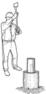
Splitting wedges (figure 11–59) are thick, heavy, metal wedges for splitting wood. The “**Splitting Wood**” section later in this chapter provides information about splitting wedges.
