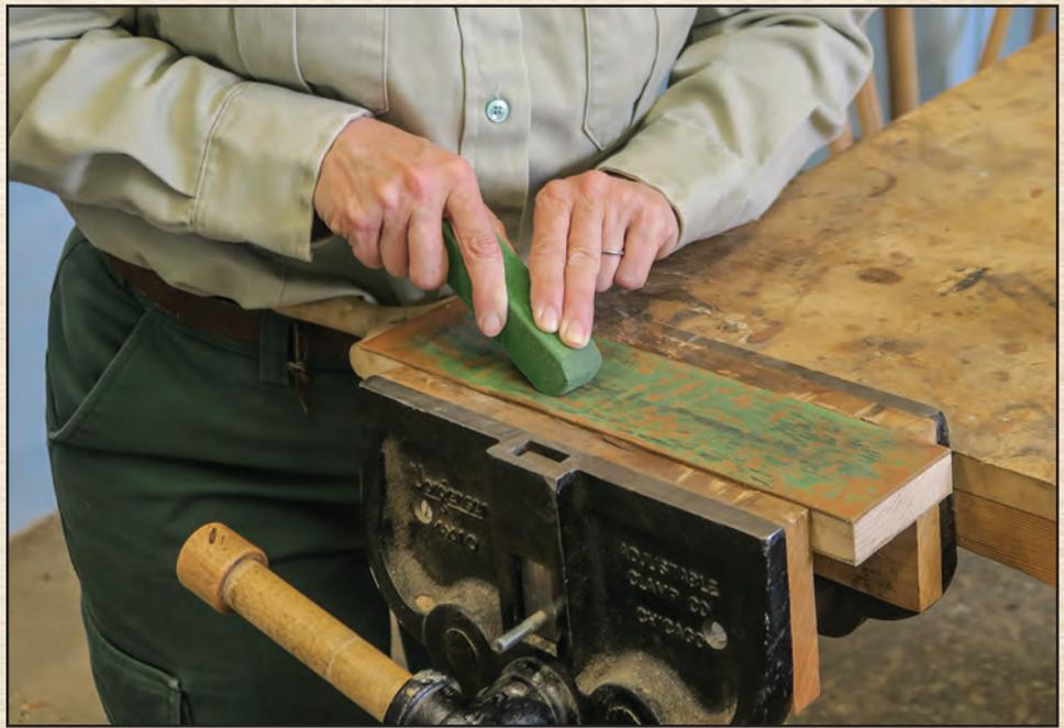
Figure 8–35—Rubbing honing compound into a leather strop attached to a board.
