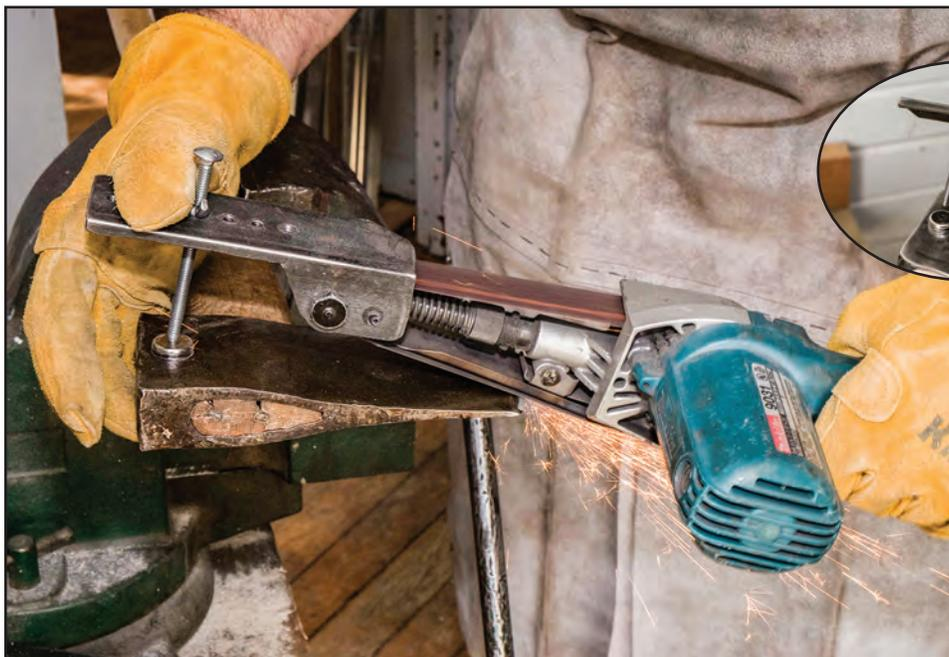
Figure 8–24—Using an electric sander to remove metal from behind the cutting edge. A rare earth magnet provides an excellent pivot point for the sanding jig (inset).
