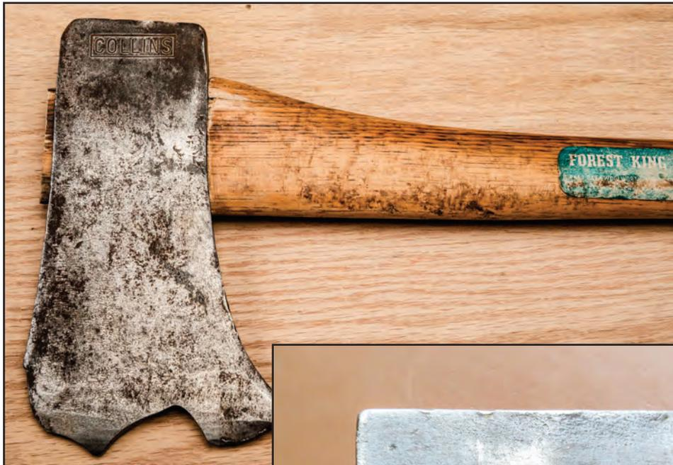
Figure 8-17—This ax had a manufacturing defect; it cannot be restored.
