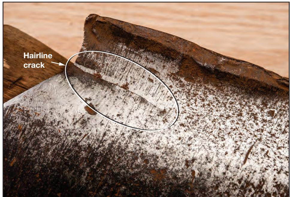
Figure 13–9—A hairline crack in an ax head.
