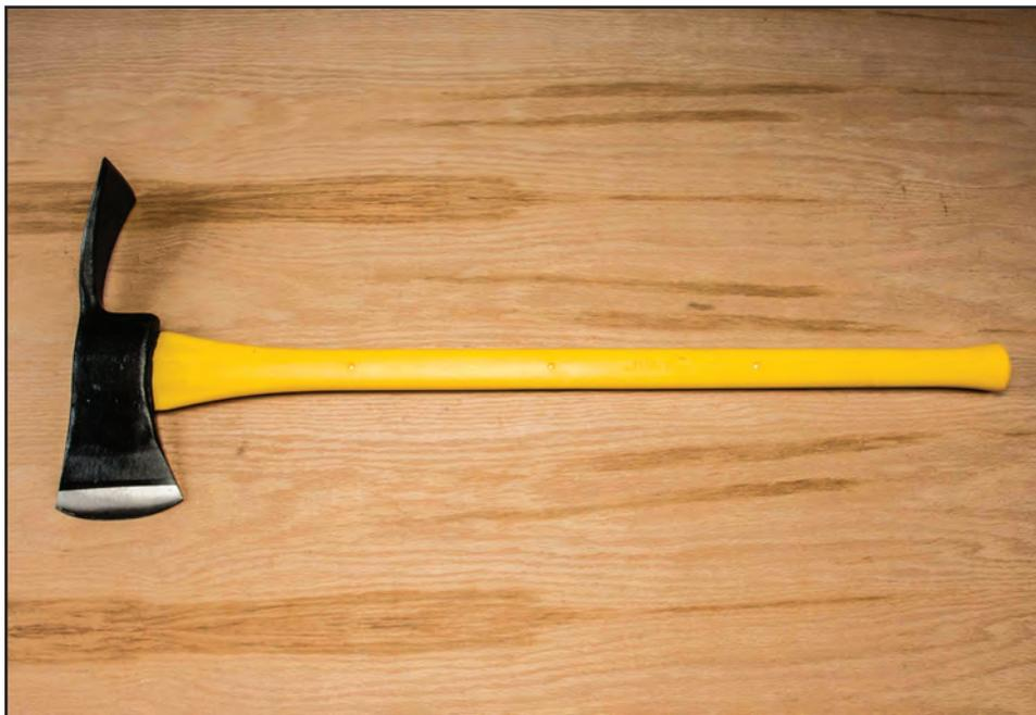
Figure 6–13—A pulaski with a synthetic handle.
