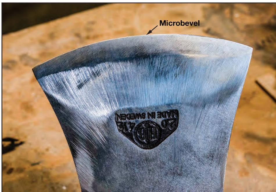
Figure 8–33—The microbevel adds strength and durability to the cutting edge.
