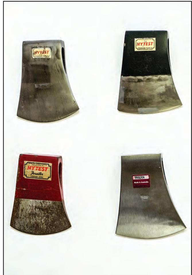
Figure 6–6—Hytest Australian-pattern ax heads.
