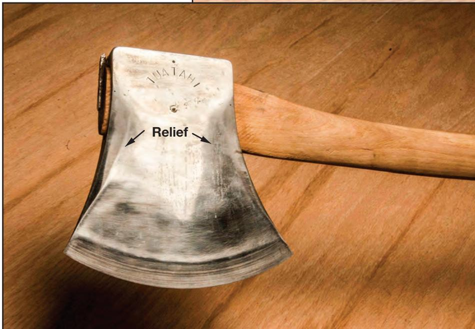
Figure 8–14—A Tuatahi competition ax showing the additional relief filed into the sides.
