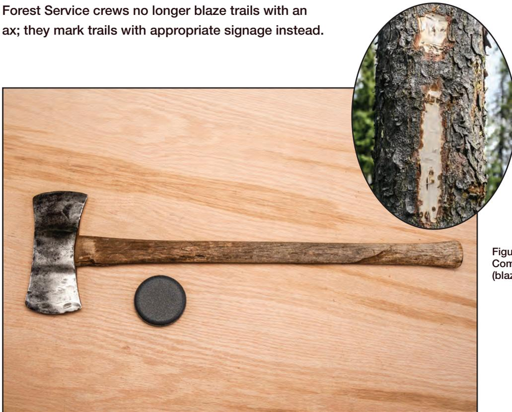
Figure 5-15—A Shapleigh Hardware Company Diamond Edge saddle (blazing) ax.
