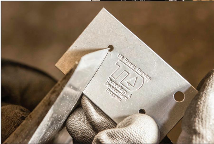
Figure 8–30—Using an ax gauge to ensure an ax head is symmetrical. Note that the tip of the cutting edge fits into the circle and the sides of the ax head are flush with the gauge.
