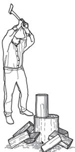
Splitting mauls and sledge hammers (figure 5-4) have hardened ends, so it is best to use one of these tools to drive metal splitting wedges or to strike other metal surfaces.
