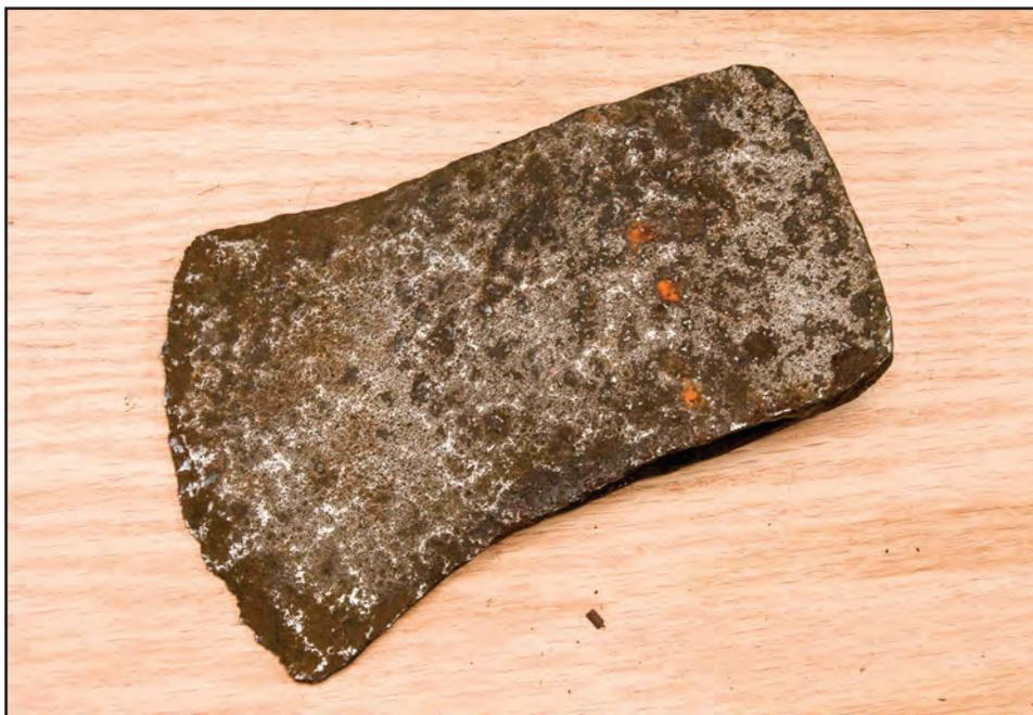
Figure 13–10—Rust and pitting on an ax head. This ax head is not worth restoring.
