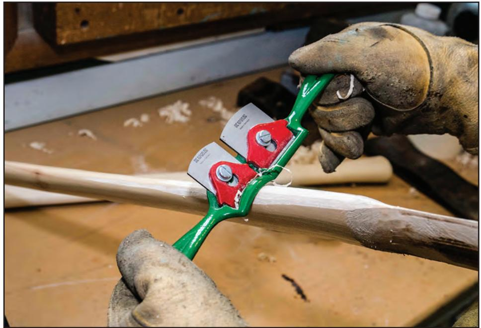
Rotate the handle regularly to keep its shape symmetrical. Some handles may be so bulky that your best option is to remove excess wood using a band saw (figure 9-7) before thinning the handle using handtools. Be careful to maintain an elliptical or flat-faced shape to the handle; a handle that is too round will pivot freely in your hands, decreasing your chopping accuracy and creating a potential safety issue.
