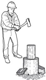
Regardless of the profile, all ax heads can get stuck in wood. The types of hollows (figure 8–13), bevels, and relief of the ax head can reduce the friction that binds it to the wood. Cutting or filing relief (figure 8–14) into the sides of an ax head reduces binding or sticking and allows the ax to more easily release from the wood.
