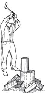
Repeat the process, alternating the wedges down the length of the log until the log splits (figure 11–81). As the split develops, it may move to a different grain. Use an ax to cut across the grain and get the split back in line with your intended cut. You can also perform this method by alternating two axes down the length of the log instead of using wedges. Using an
