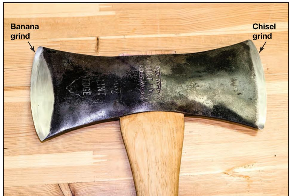
Figure 8–15—A double-bit ax with a banana grind on one cutting edge and a chisel grind on the other.
