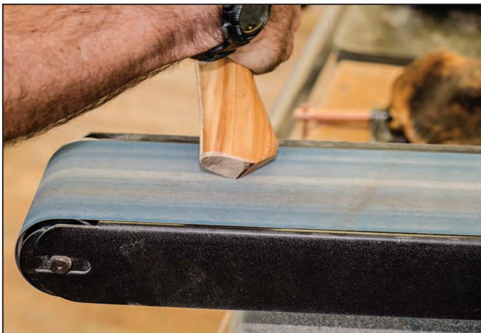
Continue rasping and seating the handle until the head fits snugly on the shoulder. Each time you place the ax head, sight down the cutting edge to ensure that it stays laterally aligned with the knob of the handle (see figure 10-3). If the alignment is to the right, remove wood from the right side of the handle that sits inside the eye (figure 10-11). If the alignment
