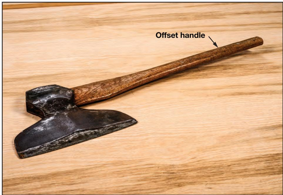
Figure 5-23—A side view of a broadax showing the offset handle.
