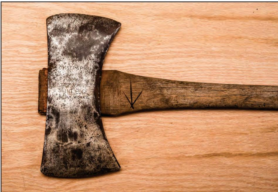
Figure 5-7—This True Temper Kelly Works Flint Edge double-bit ax (stamped “CMSTP&P RR”) has a mark on the handle that indicates the keen edge.
