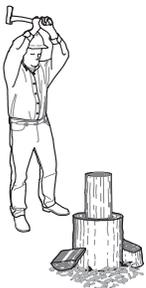
Visual inspection of single-bit ax heads may reveal a severely damaged or mushroomed poll (figure 8–19). Driving metal wedges with the nontempered poll often causes this type of damage. You may be able to grind the poll back into shape, but could lose a lot of metal and weight from the back of the ax. The poll helps provide balance and a driving force while chopping.
