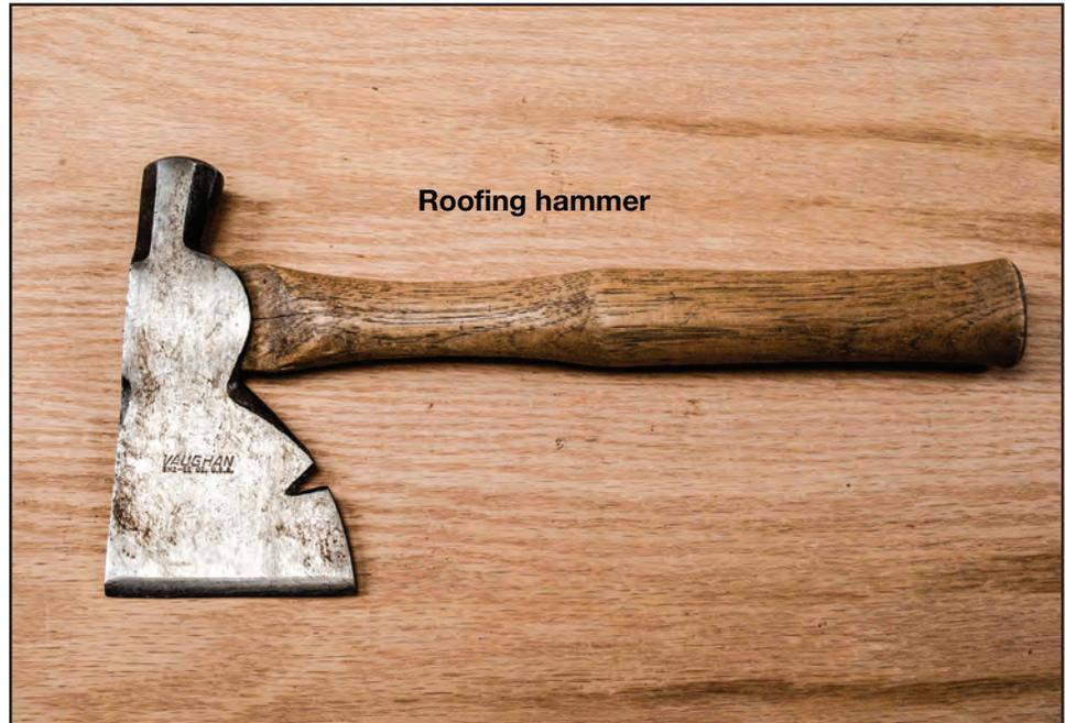
Figure 5–28—A roofing hammer (right), a fro and mallet (below), a slick (following page, top), and drawknife (following page, bottom).
