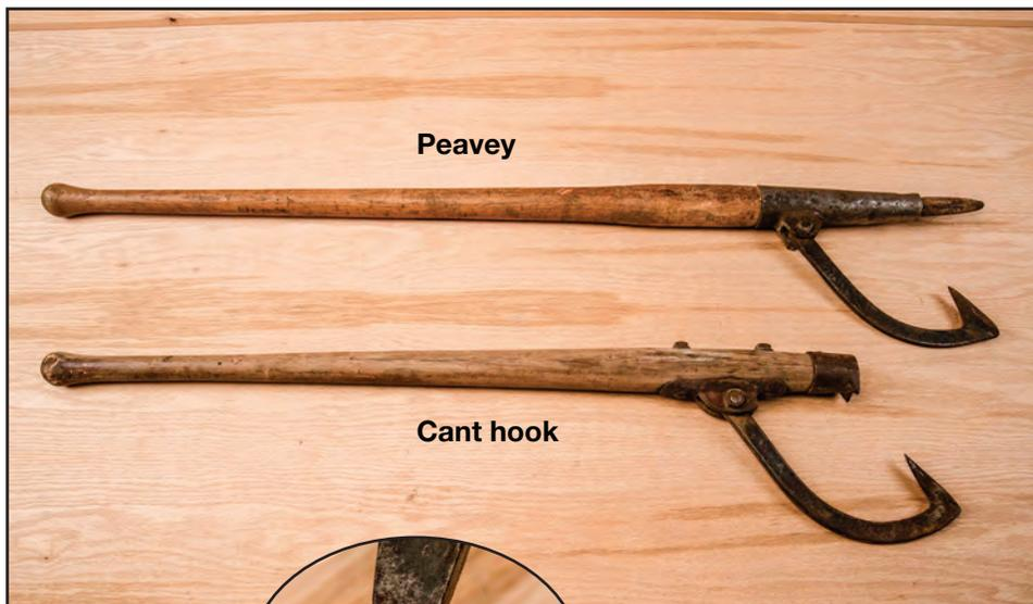
Figure 11–66—A peavey and cant hook. Note the spike on the peavey and the dogs (teeth) on the cant hook.
