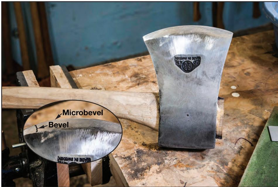
Figure 8–2—The microbevel in relation to the bevel. The inset shows a closeup view of the microbevel and bevel.
