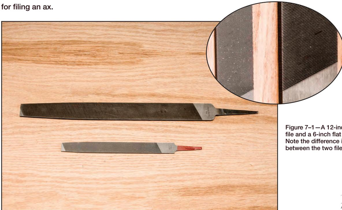
Figure 7-1—A 12-inch flat bastard file and a 6-inch flat bastard file. Note the difference in coarseness between the two files (inset).
