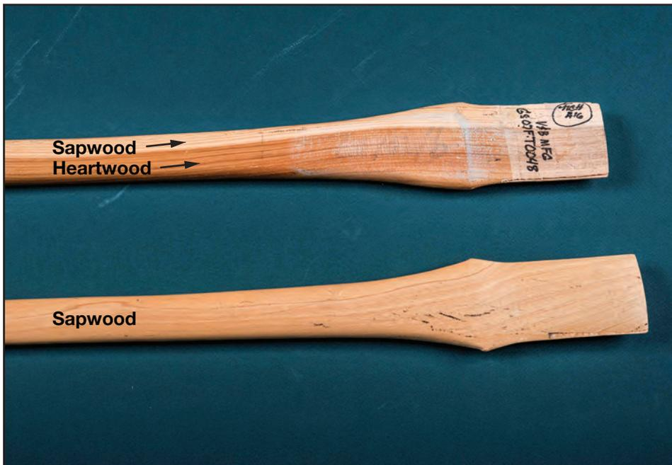
Figure 6–14—A handle containing both heartwood and sapwood (top), and a handle containing only sapwood (bottom). Research has shown that there is no difference in the strength and durability of handles containing only sapwood, only heartwood, or a combination of the two.
