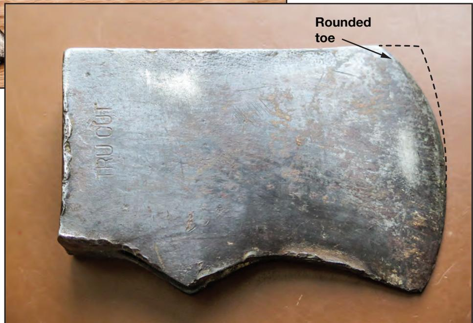
Figure 8-18—An ax head with a rounded toe.
