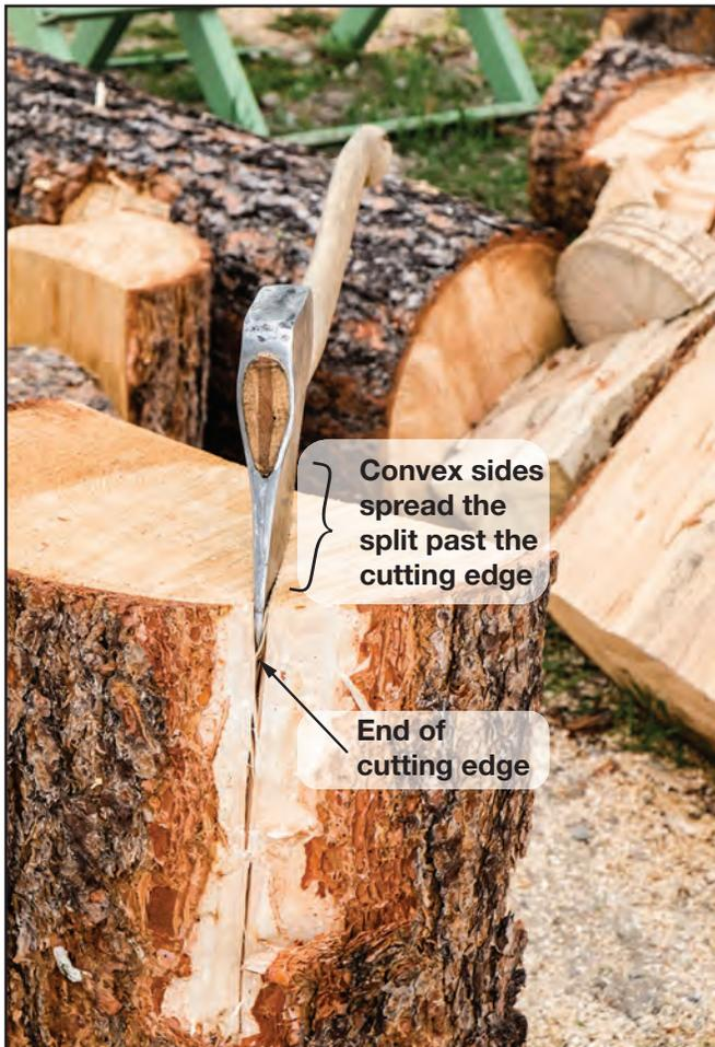
Figure 8–12—A convex head in a round of wood. Note that the sides of the ax head spread the round apart well beyond the cutting edge.
