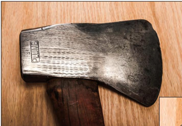
Figure 6–2—Ax heads with the weight marked on the side.
