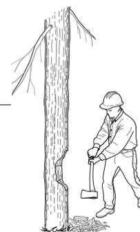
The intersection of the horizontal and the sloping cuts must line up exactly (figure 11–40). If the cuts do not line up, the tree could barber chair as it begins to fall. If you create a Dutchman in your undercut, correct it with an ax or saw before starting the back cut. The following section, “[Making the Initial Cuts,](#)” provides information about undercuts and back cuts.
