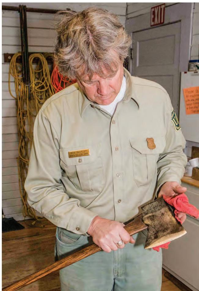
Figure 12-2—Cleaning an ax head with a rag.
