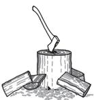
An excellent technique for making a wider notch is to chop two notches close to each other and then use the ax to remove the center portion along the grain
