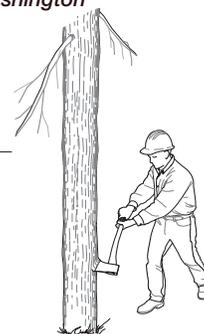
As people began to use chain saws more widely, the use of crosscut saws declined. Axes are companion tools to crosscut saws. Sawyers using crosscut saws to fell trees typically used an ax to chop out their sloping cut (figure 3-6) and to remove tree limbs. The move from crosscut saws to chain saws led to a decline in ax use.
