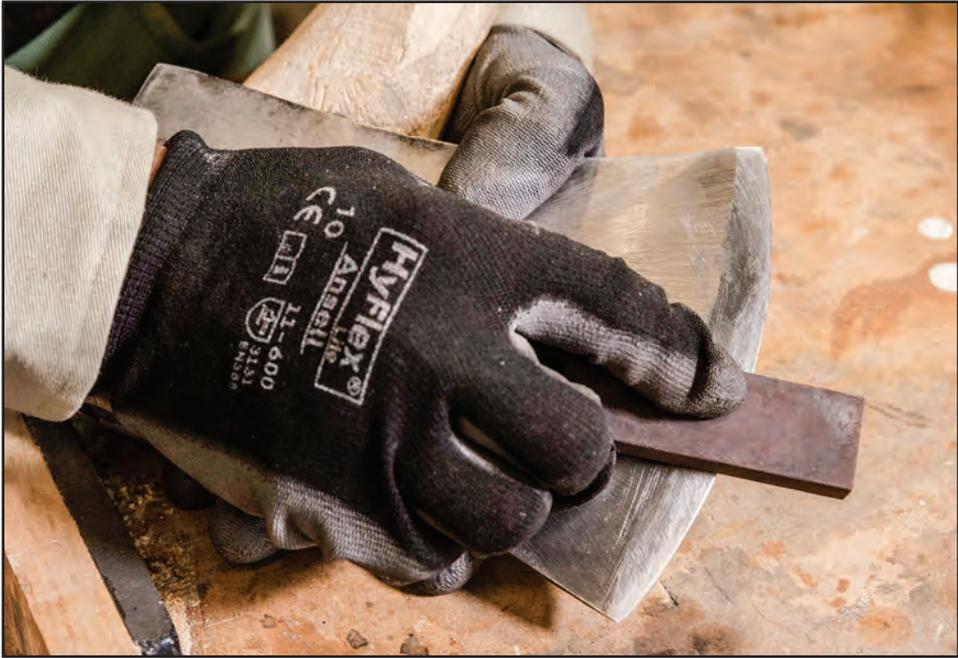
Figure 8-7—Using a whetstone to hone the microbevel.
