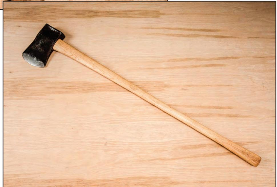
Figure 6–9—An American Axe and Tool Company splitting ax.
