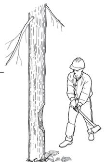
The double-bit Puget Sound felling ax is ideal for felling large-diameter trees. Figure 6–8 shows a Puget Sound felling ax with a 4-pound head on a 42-inch handle. The long, narrow blade and long handle length enable deep penetration across the breadth of large-diameter trees. The author has a similar ax head hung on a 44-inch handle, but finds the additional 2 inches of the 44-inch handle make a significant difference in the accuracy of his swings.
