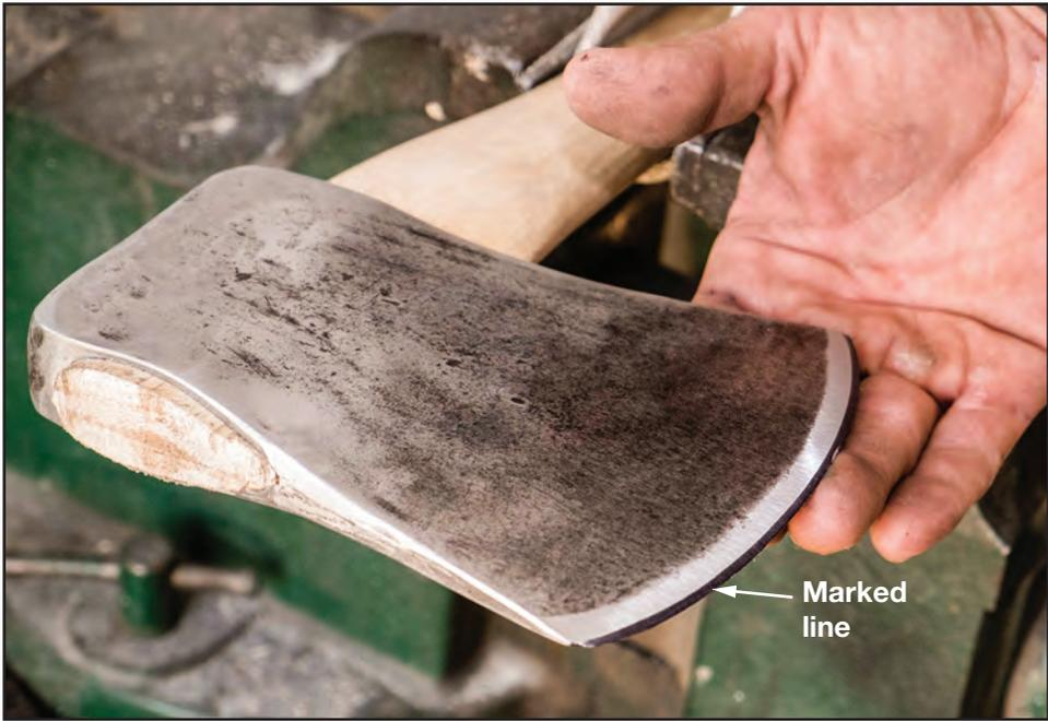
Figure 8-6—A cutting edge marked with a black felt pen. — This photo was digitally altered.
