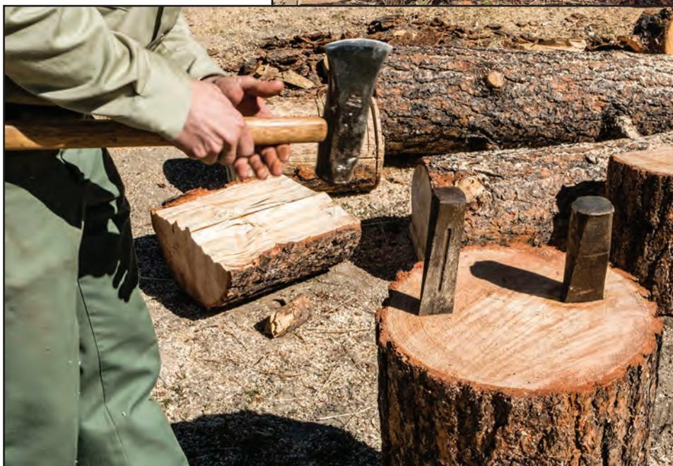
Figure 11–59—Splitting wedges.
