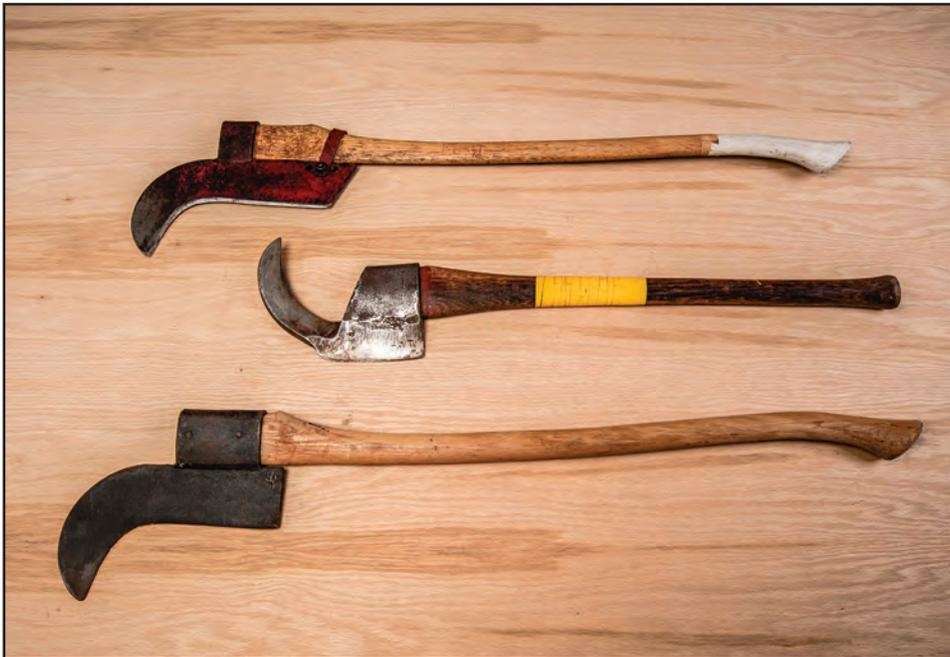
Figure 5–18—Three brush axes.
