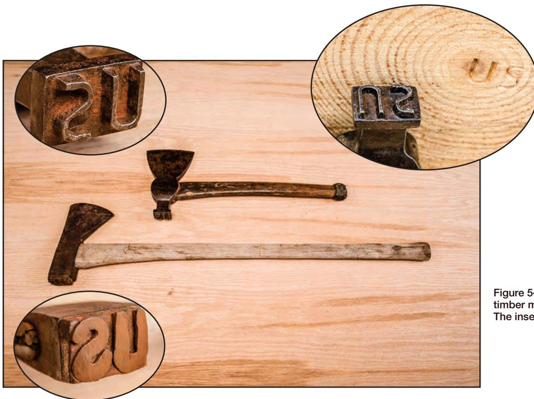
Figure 5–20—A Forest Service timber marking ax and hatchet. The insets show “US” brands.
