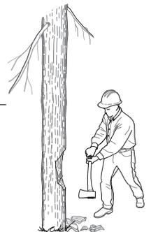
The hardened (tempered) cutting edges were durable and long-lasting. The softer center mass of the ax also provided an important feature: as the hardened steel cutting edge sank into a piece of wood, it transferred the shock of the blow into the ax head (figure 6–11). When the shock reached the cheeks of the ax, the softer metal helped absorb and dissipate the energy, reducing the amount of shock that transferred down the handle and into the axman’s hands.
