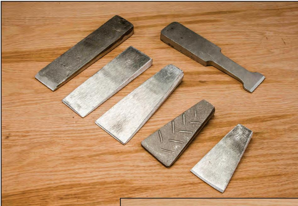
Figure 11-52—Aluminum wedges.
