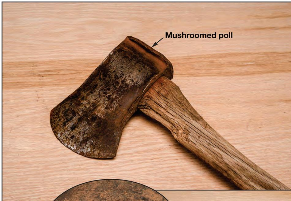
Figure 5-2—A Winchester ax with a damaged poll.
