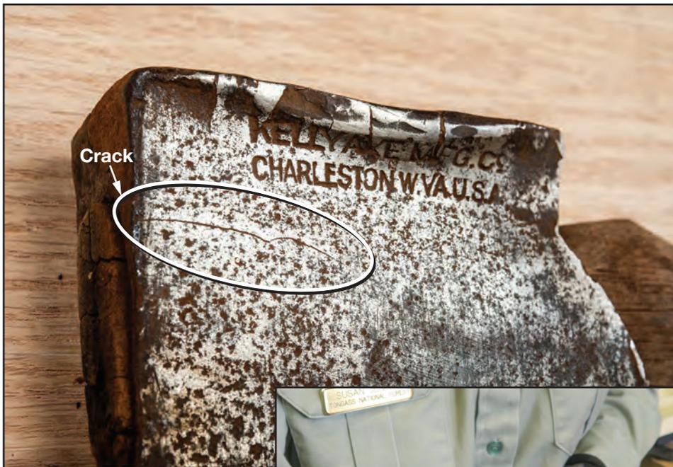
Figure 8–21—A crack in an ax head. When you see a mushroomed poll, check carefully around the eye for cracks.
