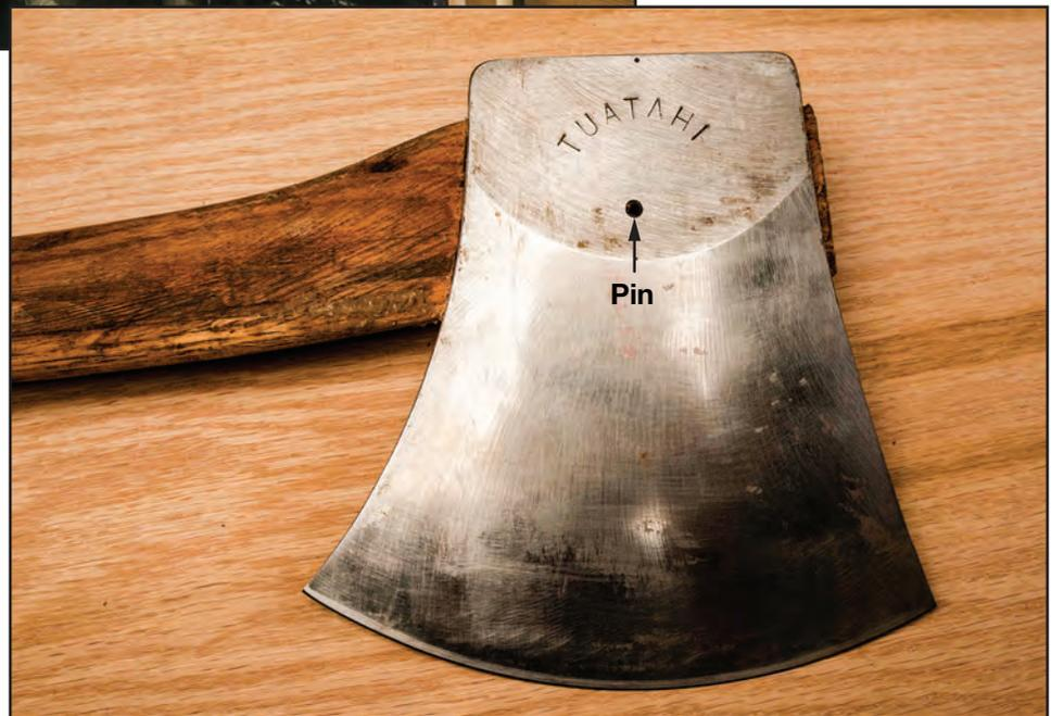
Figure 12-7—An ax head pinned to a handle.
