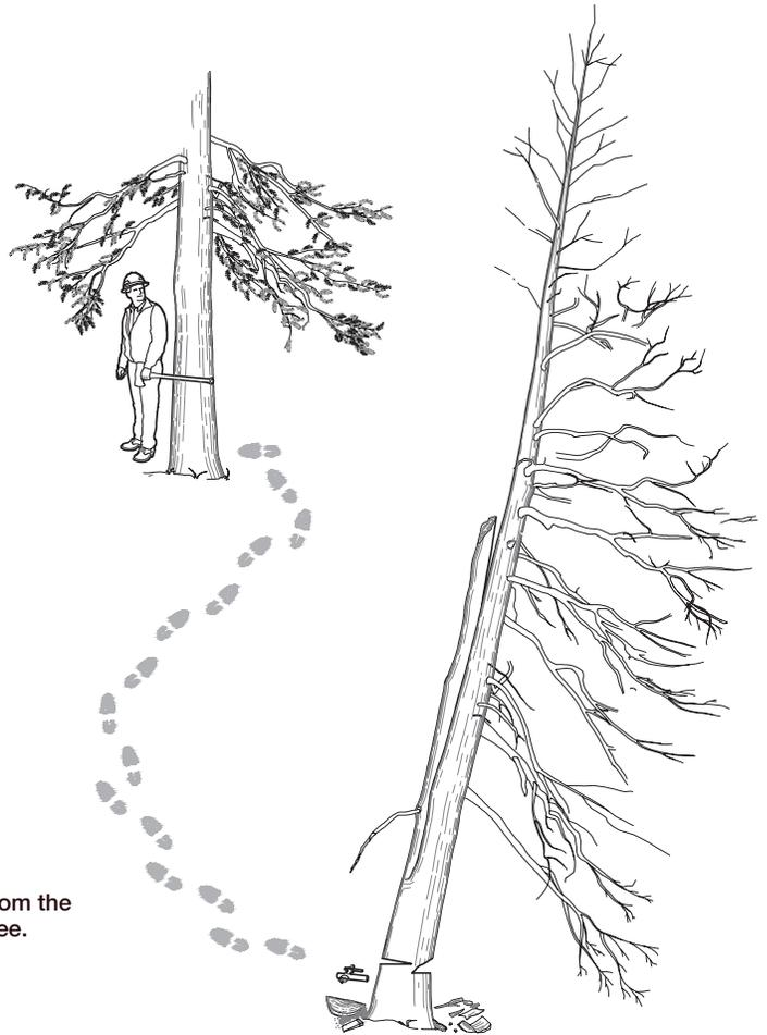
Figure 11-37—An escape path at an angle away from the back of a falling tree, but not directly behind the tree.
