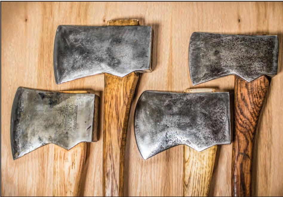
Figure 6–12—Single-bit, lugged ax patterns.
