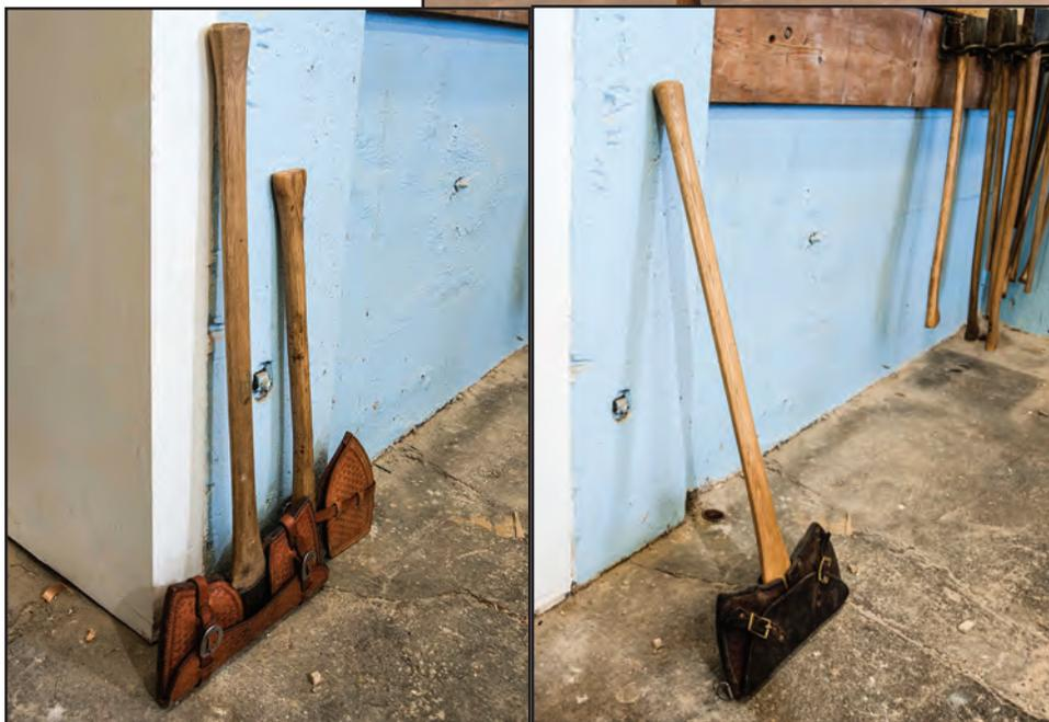
Figure 12-9—Axes leaning against a wall at roughly a 90-degree angle (left) and an ax leaning against a wall at too great an angle (right).
