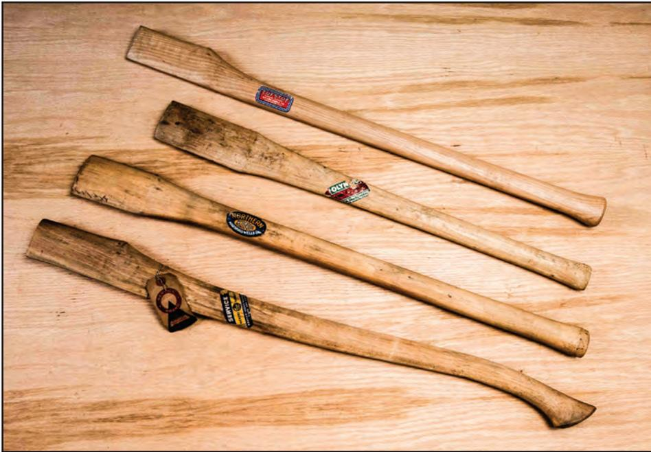
Figure 6-1—Unused old stock ax handle blanks.
