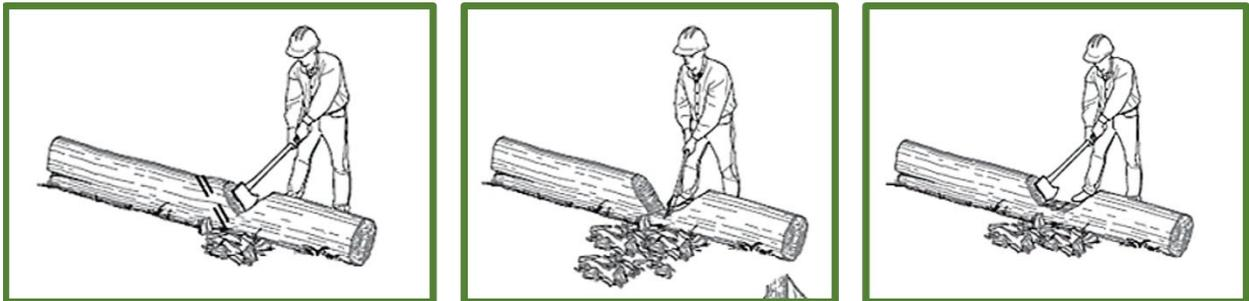
Figure 4.0.10—Connecting two faces of one notch.
