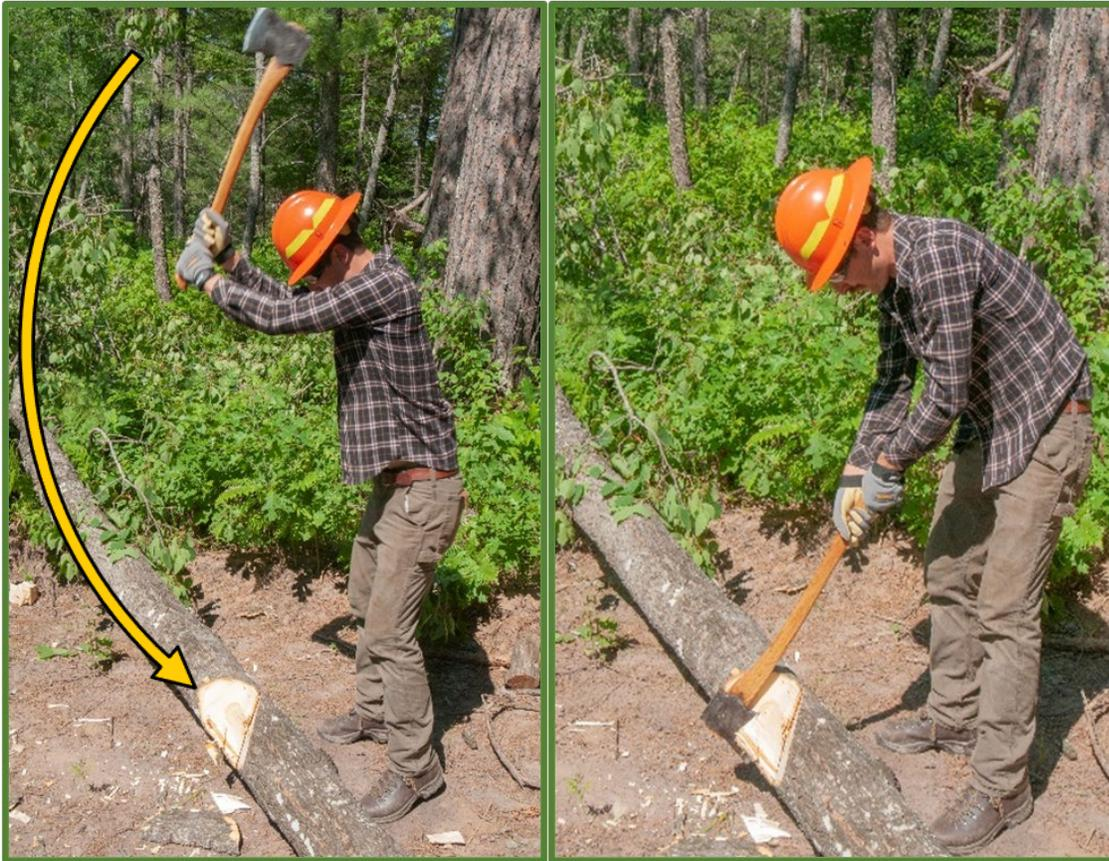
**Figure 4.0.14—Steps for an overhead chop.**
