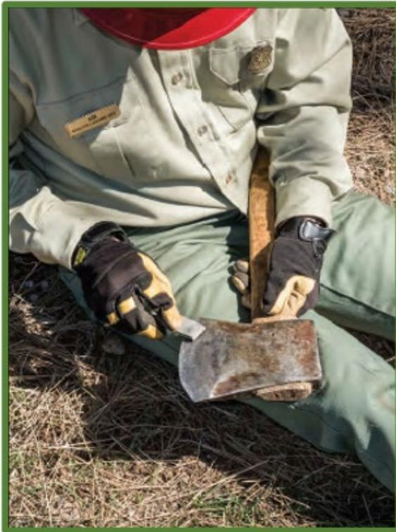
**Figure 4.0.19—Sharpen the cutting edge.**
