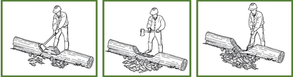
Figure 4.0.9—Connecting two separate notches.
