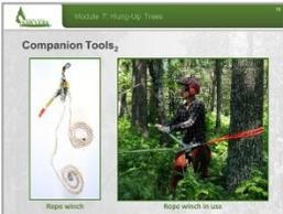
A slide titled "Companion Tools" showing a rope winch and a person using a rope winch in a forest. Each item is labeled with its name below the image.                 | <p><b>Say:</b></p> <ul style="list-style-type: none"><li>▪ <b>Rope winch:</b> A portable manual hoist with nylon rope that can lift, pull, and move lighter loads across great distances.</li></ul> <p><b>DISPLAY NEXT SLIDE</b></p>
